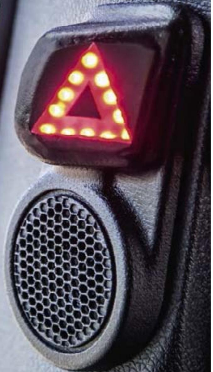
**Sending an important signal: Blind Spot Assist warns drivers of the presence of other road users when the truck makes a turn. The system is yet another milestone on the "road to accident-free driving."**
